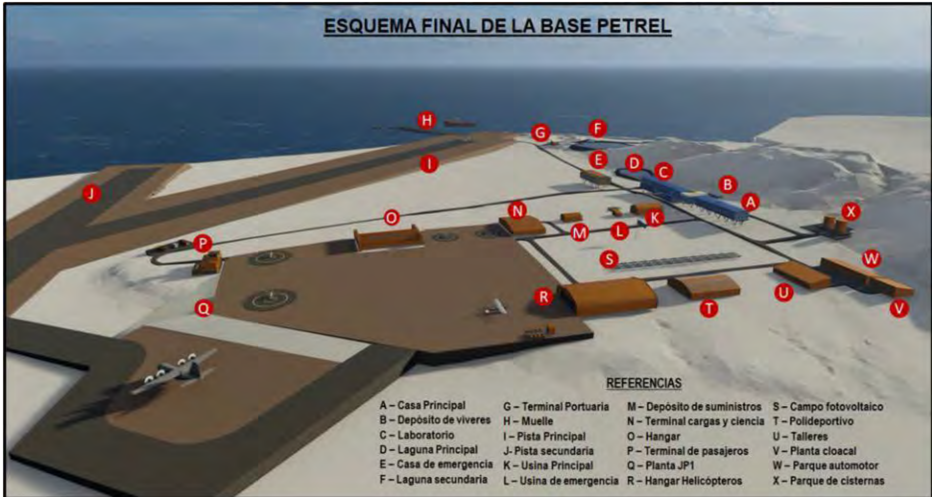
Figure 37: General outline of the initial proposal for the new Petrel Base (the quay was excluded in the analysis of alternatives).
