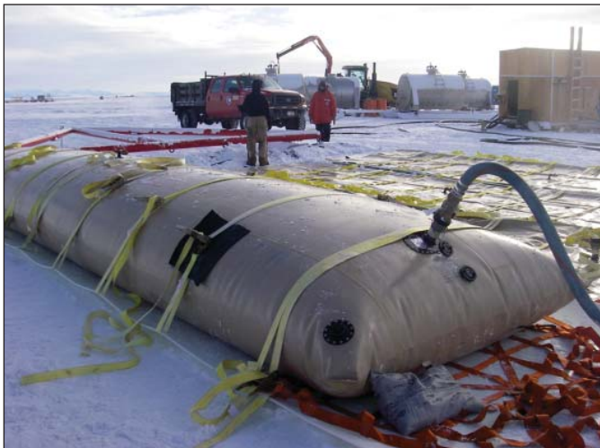
Figure 20. shows an image of the proposed flexible bulk fuel container on a skid base.
